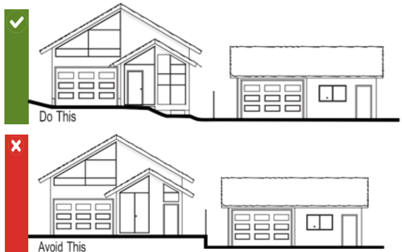
Figure 2: Building with the slope vs. re-grading
